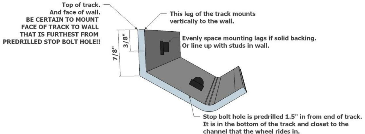
*Note you want track installed level, but floor may not be level. Verify height points from floor along full length of track to be sure you have proper clearance. Keep track level and raise height if need be to get clearance. Also be sure that floor guide will reach door properly after setting height of track.*
