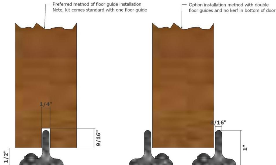
If you want the alternative option shown in picture with double guides, be sure to order an extra floor guide. Otherwise cut a 1/4" wide kerf centered in bottom of door. To determine depth of kerf cut, subtract desired gap under door from 1" and add 1/16", so for a 1/2" gap under door you would have a 1/4" wide and 9/16" deep slot/ kerf. This is easiest to do with a router and a slot cutter.
